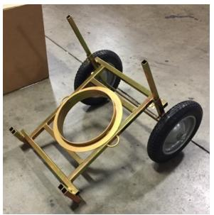
Install the tall square tubing section into the main frame and secure with the cast wing bolts. Then slide the round axle through the tubing and install the wheels. Secure the wheels in place with the washer and cotter pin.
